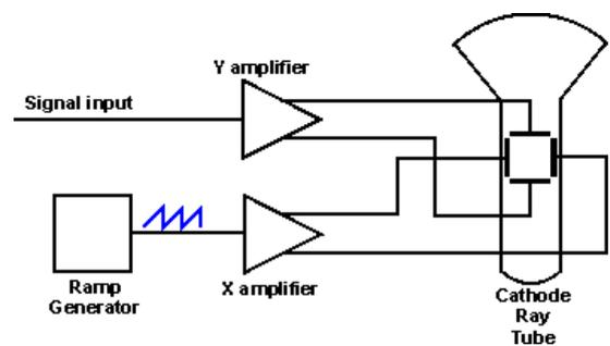
The cathode ray tubes use electrostatic deflection to cause the electron beam position and hence the trace position to change. This method rather than the electromagnetic deflection system used in many CRT based television sets is used to ensure that a sufficiently high speed of operation is attained. The magnetic deflection used in televisions does not enable the very high speeds needed for oscilloscopes to be achieved.
