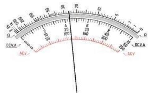
Resistance measurements, in particular, are of low precision due to the typical resistance measurement circuit which compresses the scale heavily at the higher resistance values. Inexpensive analog meters may have only a single resistance scale, seriously restricting the range of precise measurements. Typically an analog meter will have a panel adjustment to set the zero-ohms calibration of the meter, to compensate for the varying voltage of the meter battery.
