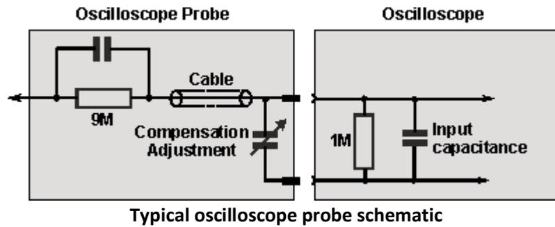
Typical oscilloscope probe schematic
