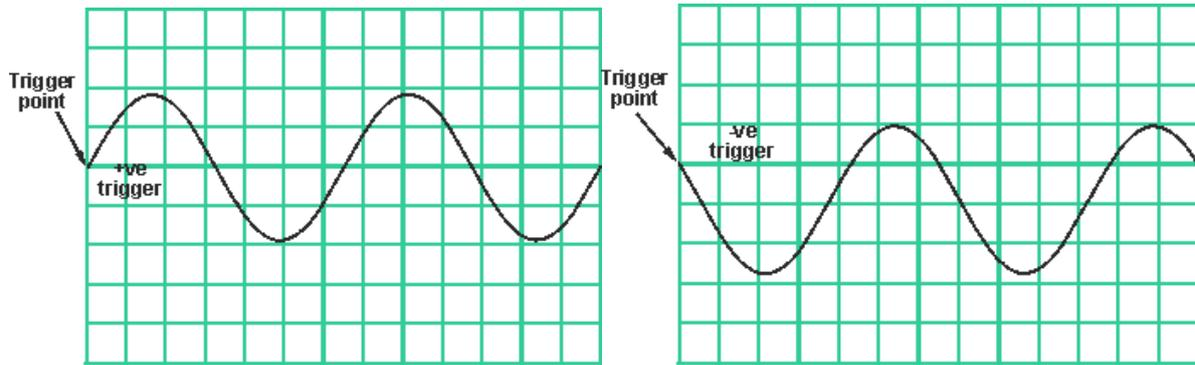
As can be seen, the setting of both the oscilloscope trigger levels and slope determine the image that is seen on the screen. Careful adjustment of both controls ensures that the required portion of the waveform is seen.
