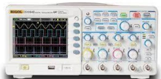
While it is useful to display a single waveform, many measurements and measurement techniques require more than one waveform to be displayed at any one time. This can be used to compare waveforms and look at how different waveforms interact or when events occur on more than one waveform. Many dual channel or multi-channel oscilloscopes exist that allow two or more waveforms to be displayed at the same time.
