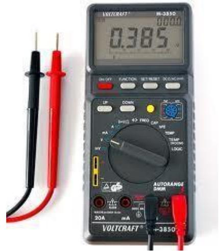
A multimeter can be a hand-held device useful for basic fault finding and field service work, or a bench instrument which can measure to a very high degree of accuracy. They can be used to troubleshoot electrical problems in a wide array of industrial and household devices such as electronic equipment, motor controls, domestic appliances, power supplies, and wiring systems.
