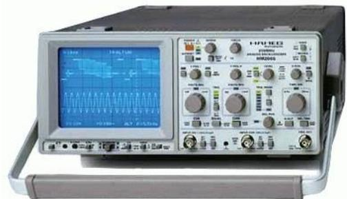
The key to the operation of an analog scope is its display. It uses the cathode ray tube or CRT. This form of display was for many years the only viable form of display that could be used to display images. Accordingly it was used in television sets for many years, although other forms of display including LCDs, LEDs and many other format are now used, but these all require digital signal inputs to the display.
