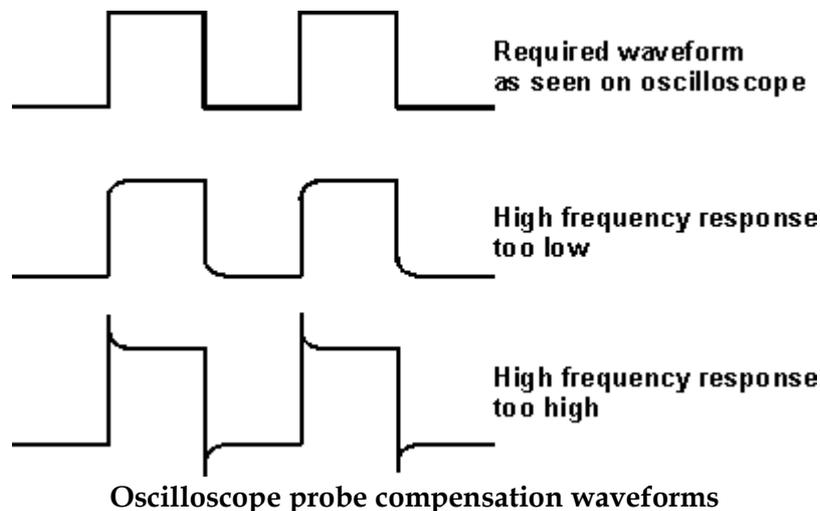
Oscilloscope probe compensation waveforms
