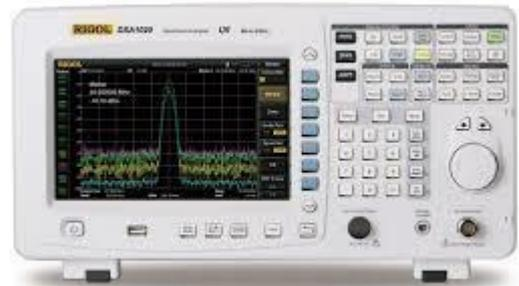
Essentially a spectrum analyser scans a band of frequencies set by the user, and notes the signal levels, displaying them on a screen. In this way it is possible to obtain a plot of the signals appearing in any band of frequencies.
