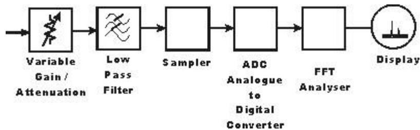
The FFT spectrum analyzer can be considered to comprise of a number of different blocks:
