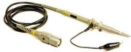
**Oscilloscope probe** Scope probes are generally classified according to the level of attenuation of the signal they provide. Types including 1X (giving a 1 : 1 attenuation ratio), 10X (giving a 10 : 1 attenuation ratio) and 100X (giving a 100 : 1 attenuation ratio) are available:
