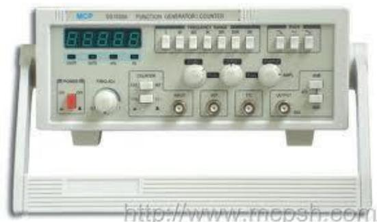
instrument that is able to meet most user needs, while remaining simple and easy to use. Maximum frequencies: The analogue function generators do not have the high frequency limitations on nonsinusoidal waveforms such as triangles and ramps as do the digital function generators.
