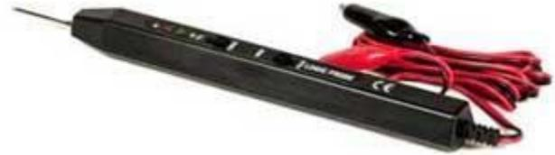
This makes logic probes very portable and easy to use for troubleshooting and general simple maintenance work on low complexity logic circuitry.
