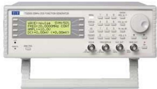
In addition to producing sine waves, function generators may typically produce other repetitive waveforms including sawtooth and triangular waveforms, square waves, and pulses. Another feature included on many function generators is the ability to add a DC offset.
