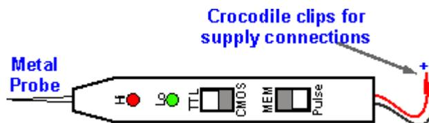
The first requirement before using the logic probe is to connect the power connections to the circuit. Apart from ensuring they are the right voltage, the points used for connecting the crocodile clips to should be accessible and provide a reliable connection without the risk of touching any adjacent components or other connections.
