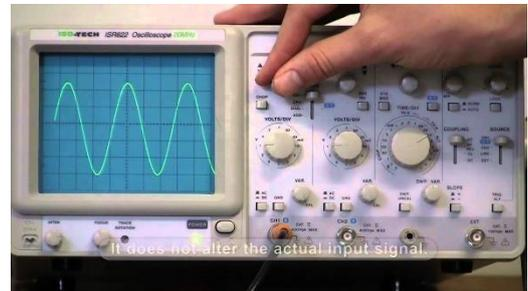
Checking the resolution within the oscilloscope specification will ensure that the instrument will offer the correct dynamic range and resolution.
