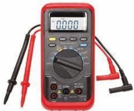
Any ammeter, including a multimeter in a current range, has a certain resistance. Most multimeters inherently measure voltage, and pass a current to be measured through a shunt resistance, measuring the voltage developed across it. The voltage drop is known as the burden voltage, specified in volts per ampere. The value can change depending on the range the meter selects, since different ranges usually use different shunt resistors.
