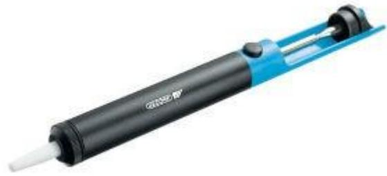
While a little more expensive than desoldering braid, desoldering pumps last considerably longer. Indeed, really the only part of the pump that may be worn by the desoldering process is the pump nozzle, due to the repetitive application of the heat of soldering, which nevertheless will have an operating life of many thousands of operations. Most desoldering pumps have replaceable nozzle, so even if the nozzle is worn, the pump is not necessarily written off.
