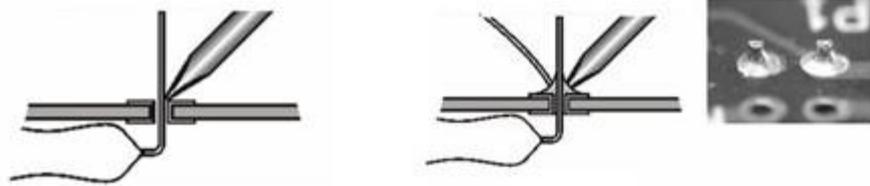
The quantity of solder that we must use must be that much, in order our terminal to be covered evenly all around, without being too much and appear as a marble, but not insufficient either, so that in some points not to be a joint between the terminal and the pad.
